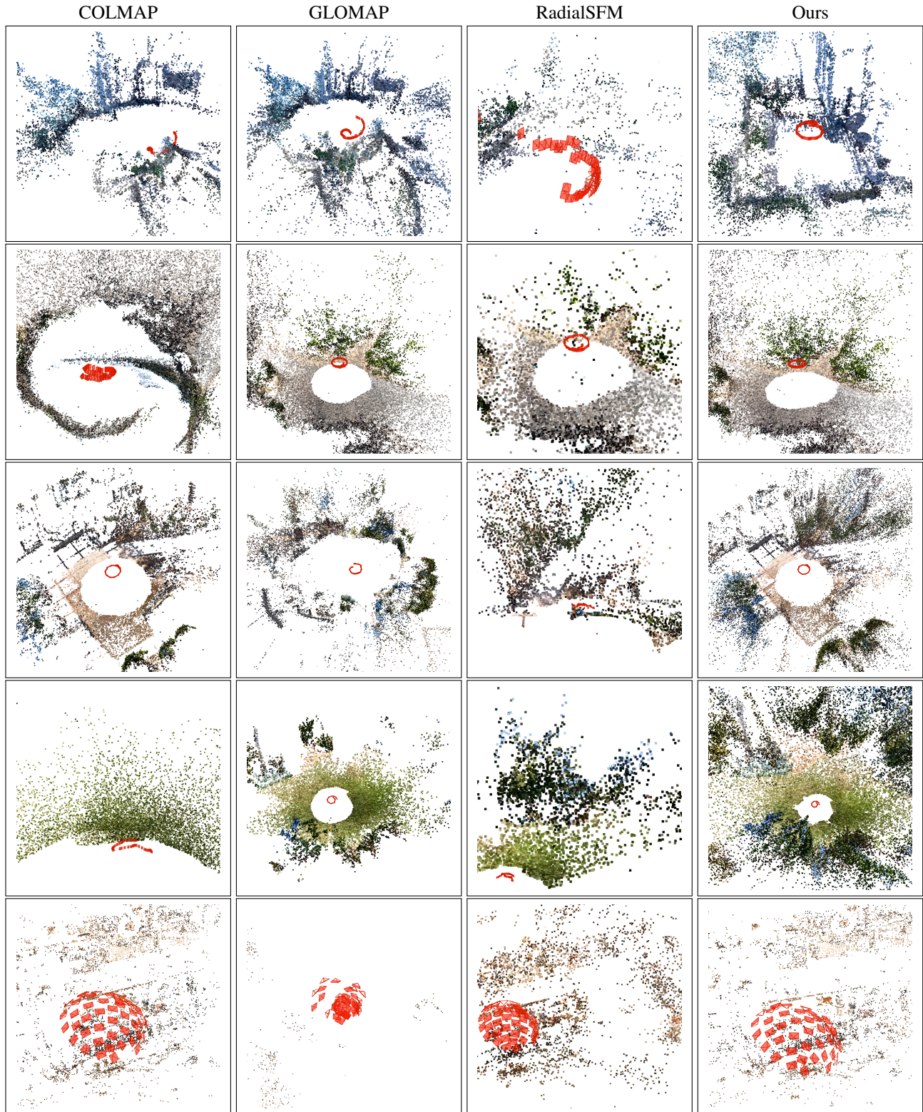
Figure 4. Example reconstruction results. COLMAP, GLOMAP and RadialSFM exhibit many failed reconstructions, where often the camera motion is incorrectly interpreted as inward-facing instead of outward-facing. In contrast, our method reliably reconstructs these scenes. From top to bottom: iPhone 13 scenes deck and ocean and Nexus 5X scenes arboretum7 and education1 from the PhoneSweep dataset; scene 01_Welder from the Deep View Video dataset.
