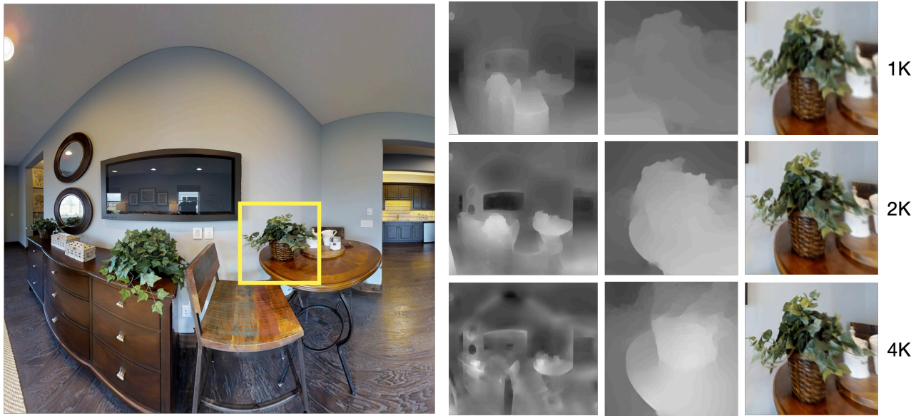
Figure 9: Comparison of generated depth maps and view synthesis at various resolutions. At lower resolutions, the depth map lacks detail, but at higher resolutions, the depth map lacks global coherence and artifacts are introduced. Left : Input image (cropped to fit page) with detail region outlined in yellow. Right : Generated depth maps, depth map detail, and view synthesis detail, at 512 \times 1024 ( top ), 1024 \times 2048 ( middle ), and 2048 \times 4096 ( bottom ) input image resolution. Image from Matterport3D dataset [5].
